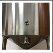
Place the cap cover stopper into the hole of thermowell, then insert the thermometer.
